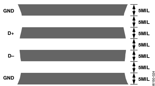
Figure 24. Typical Arrangement of Signal Tracks
